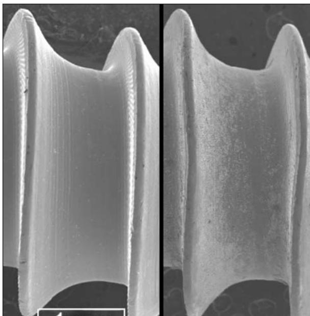
Figure 4—Photomicrograph of 2 threads for comparison of an untreated control screw (left) and 8.5 GW/cm<sup>2</sup> treated screw (right). Notice the irregular contour of the threads on the treated screw, which is consistent with moderate thread damage. Bar = 1 mm.
