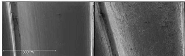
Figure 3—Photomicrograph used for comparison of the surface on an untreated control screw (left) with a similar peened area on an 8.5 GW/cm<sup>2</sup> treated screw (right). The surfaces were evaluated for elevations and pits. Bar = 800 μm.
