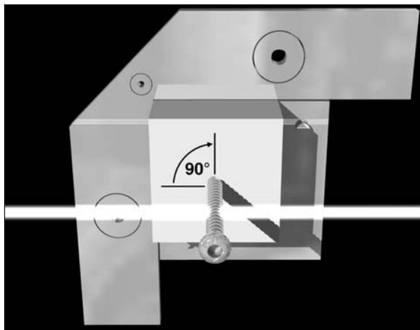
Figure 1—A drawing of a screw partially embedded in the Teflon block that is mounted in the robotic work arm. Simultaneous laser pulses are seen striking the screw on opposite sides. After these 2 laser pulses strike the screw, the construct was rotated 90° and treated again similarly by an additional 2 laser pulses.
