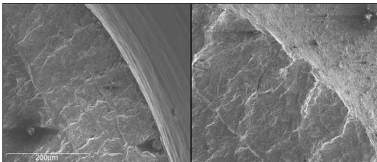
Figure 5—Photomicrograph used for comparison of the fractured ends at the point of crack initiation of an untreated control screw (left) and an 8.5 GW/cm<sup>2</sup> treated screw (right). Notice the irregularity of the surface on the 8.5 GW/cm<sup>2</sup> treated screw (right), compared with the control screw (left). Bar = 200 µm.
