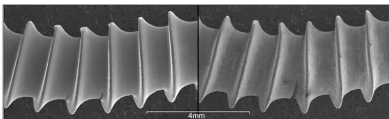
Figure 2—Photomicrograph of the failure site of an untreated control screw (left) and 6 gigawatt (GW)/cm<sup>2</sup> treated screw (right) after mechanical testing. Two cracks are seen on the control screw (left) and 1 on the 6 GW/cm<sup>2</sup> treated screw (right). Bar = 4 mm.
